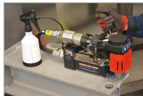
Through spindle cooling system
