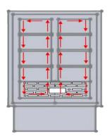
A chimney effect that drives air upward along the center support bar, together with the oven's rectangle shape and vented shelving, allows for exceptional heat flow pattern MODEL: FE50SS /50kg FE100SS/100kg FE150SS/150kg FE200SS/200kg
